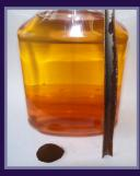
will occur. Phase separation dramatically lowers the octane and oxygenate levels in fuels resulting in very poor running engines, O2 sensor/catalytic converter failures, and serious engine damage.
